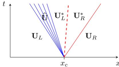
FIGURE A1 Structure of the solution for the Riemann problem for the state [Color figure can be viewed at wileyonlinelibrary.com]
