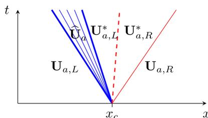
FIGURE A2 Structure of the solution for the Riemann problem for the sensitivity [Color figure can be viewed at wileyonlinelibrary.com]
